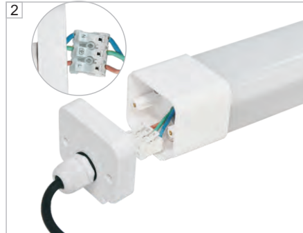
Open the end cap and insert your local cable to terminals as per corresponding cable marks
