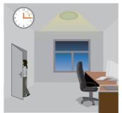
Light will dim to 10%/20%/30%/50%(options) after the hold time when no movement in detection area
